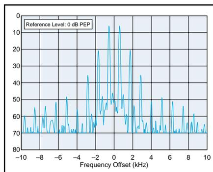
**Figure 2—Worst-case VHF/UHF spectral display of the TS-2000 transmitter during two-tone intermodulation distortion (IMD) testing. The worst-case third-order product is approximately 22 dB below PEP output, and the worst-case fifth-order product is down approximately 36 dB. The transceiver was being operated at 100 W PEP output at 50.2 MHz.**
