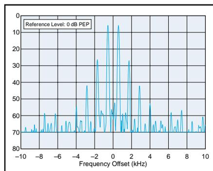
**Figure 1—Worst-case HF spectral display of the TS-2000 transmitter during two-tone intermodulation distortion (IMD) testing. The worst-case third-order product is approximately 27 dB below PEP output, and the worst-case fifth-order product is down approximately 42 dB. The transceiver was being operated at 100 W PEP output at 1.85 MHz.**
