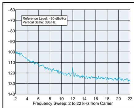
**Figure 5—Worst-case VHF/UHF spectral display of the TS-2000 transmitter output during composite-noise testing. Power output is 50 W at 430.02 MHz. The carrier, off the left edge of the plot, is not shown. This plot shows composite transmitted noise 2 to 22 kHz from the carrier.**
