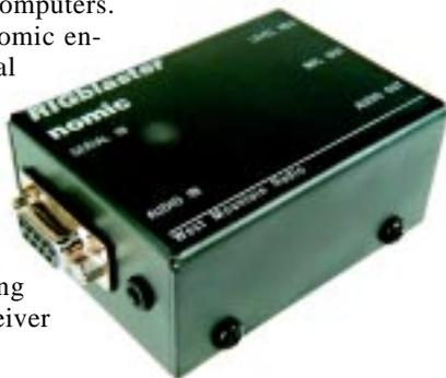
are made through a RJ45 modular telephone-style jack on the right side of the Nomic. This jack is labeled **MIC OUT**, but it doesn’t necessarily need to be connected to your transceiver microphone jack. You can just as easily make the connection to the auxiliary jack.
