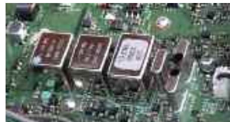
PHOTO 6: 2nd IF roofing filters.
