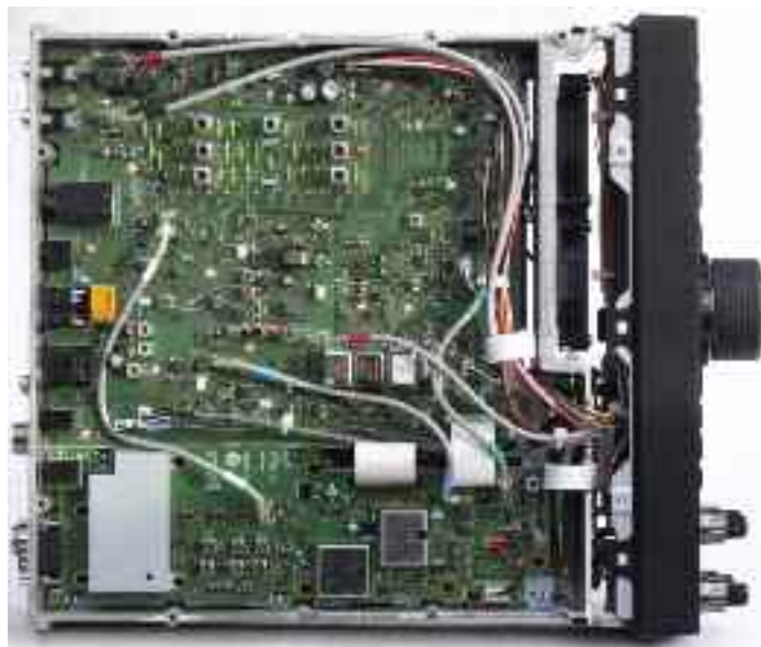
PHOTO 3: Underneath view showing signal processing boards.
